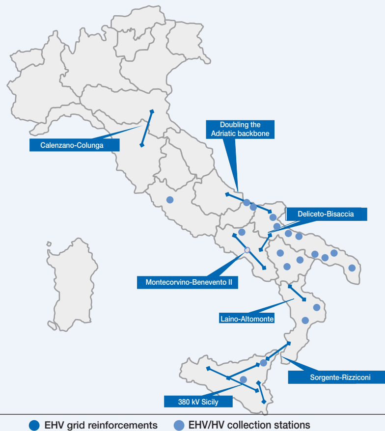
Figure 2 - Main action on the 380 kV grid needed to make full use of energy produced by renewable source systems
