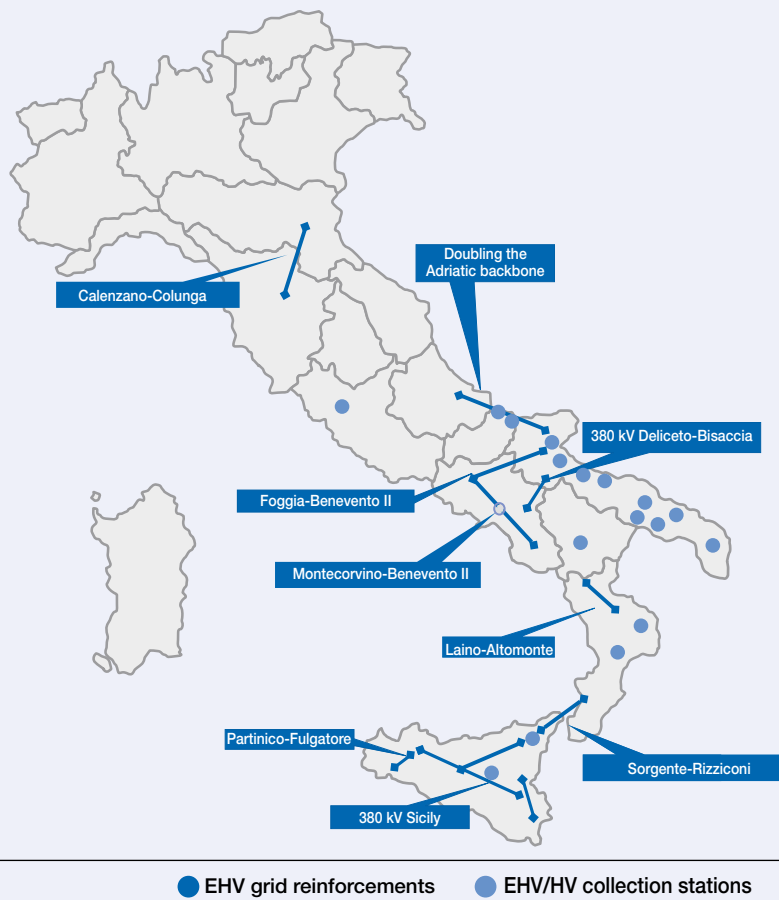
Figure 2 - Main action on the 380 kV grid needed to make full use of energy produced by renewable source systems
